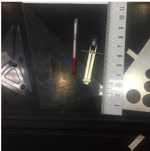
**Figure 2. Photo of measuring tools used which have been adapted with tactile markings to be accessible to blind users. Photo taken by Natalie Shaheen and used with permission.**
